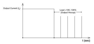
It is not recommended to prolong the duration of  $I_0$  when it is <105~175% but >100%, since it may cause damage to the PSU.
