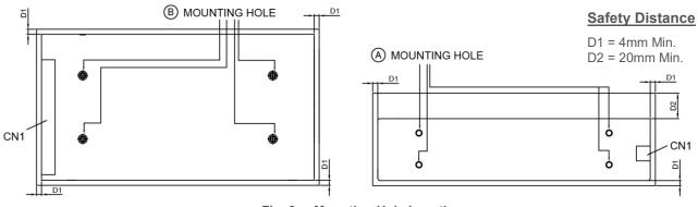
Fig. 3 Mounting Hole Locations
