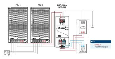
Fig. 5 Redundancy Operation Connection Diagram
