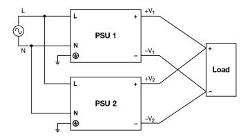
Fig. 6 Parallel Operation Connection Diagram
