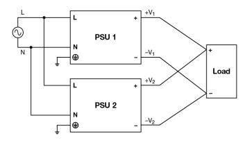
Fig. 6 Parallel Operation Connection Diagram
