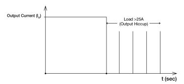
It is not recommended to prolong the duration of  $I_0$  when it is <25A but >14.6A, since it may cause damage to the PSU.
