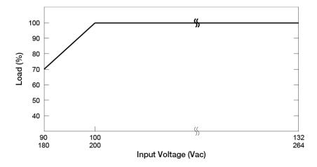
No output power de-rating for the input voltage from 100 Vac to 132 Vac & 200 Vac to 264 Vac
