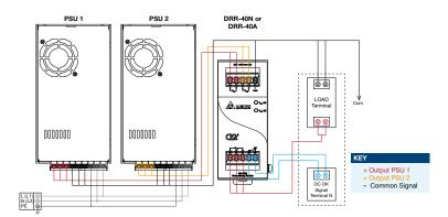
Fig. 5 Redundant Operation Connection Diagram
