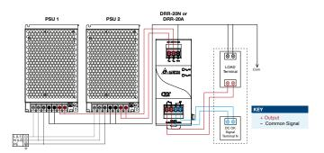
Fig. 5 Redundancy Operation Connection Diagram
