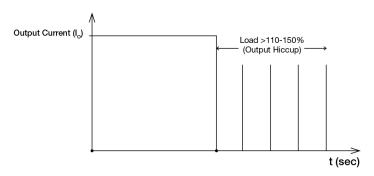
It is not recommended to prolong the duration of  $I_0$  when it is <110-150% but >100%, since it may cause damage to the PSU.
