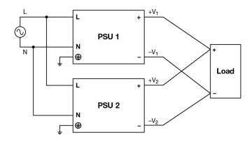
Fig. 6 Parallel Operation Connection Diagram
