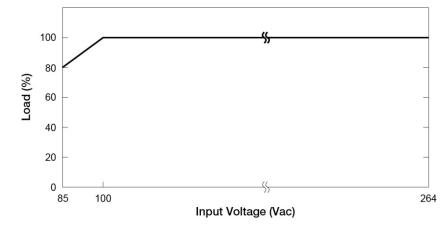
No output power de-rating for the input voltage from 100 Vac to 264 Vac
