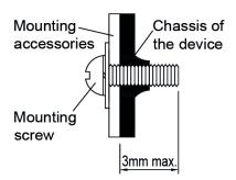
■ For PMT and PML Series (Refer to Fig. 4): Only use M3 screw ≤ 3 mm (0.20 inch) through the base mounting holes. This is to keep a safe distance between the screw and internal components. Recommended mounting tightening torque: 4~7 Kgf.cm.
