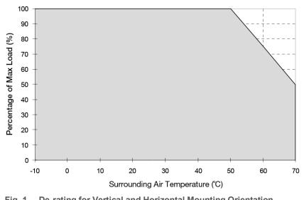
Fig. 1 De-rating for Vertical and Horizontal Mounting Orientation > 50°C de-rate power by 2.5% / °C
