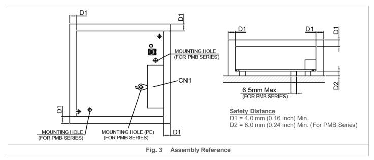
Ensure the mounted device is kept at  $\geq$  4 mm (0.16 inch) safety distance at all sides from other components and equipments. In addition, to ensure sufficient convection cooling, always maintain a distance of  $\geq$  20 mm (0.79 inch) from ventilated surfaces while the device is in operation.
